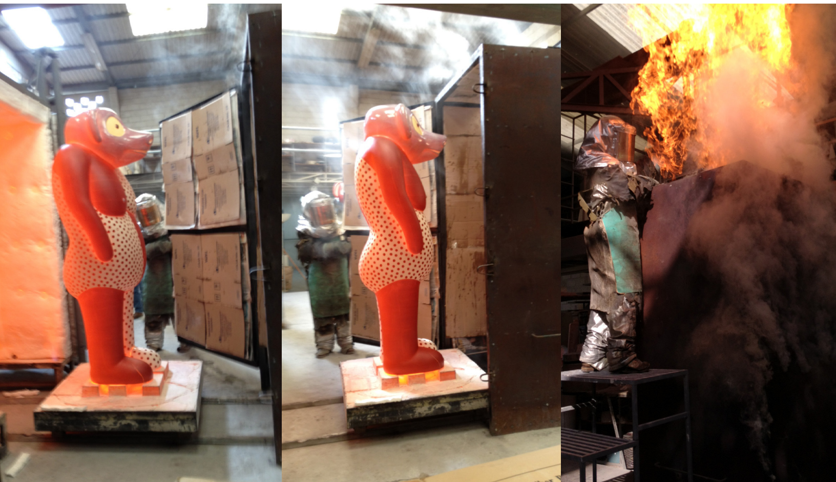
A glowing hot Tanuki exiting the kiln and being enclosed in a chamber lined with combustible materials
